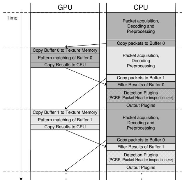
Figure 4: Execution flow of a single CPU process.
