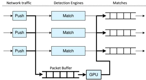
Figure 2: Batching different flows to a single buffer.
