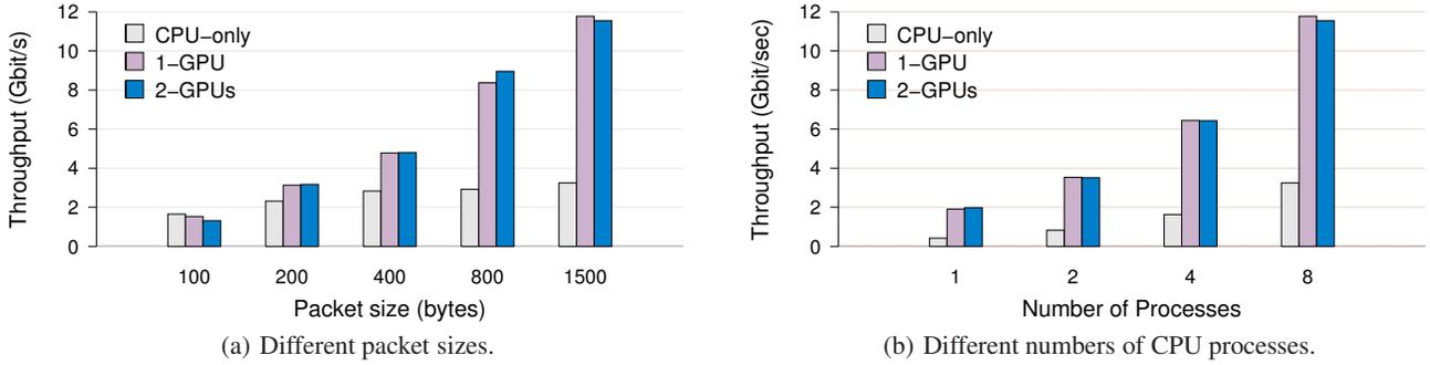
Figure 10: Overall sustained throughput for different workloads and configurations.
