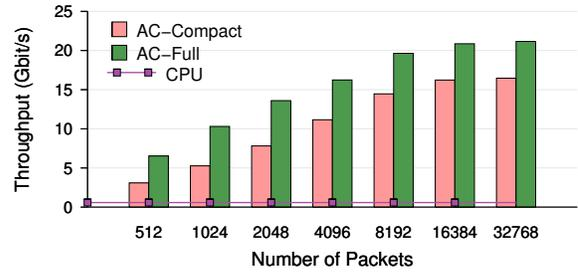
Figure 8: GPU throughput for AC-Full and AC-Compact.
