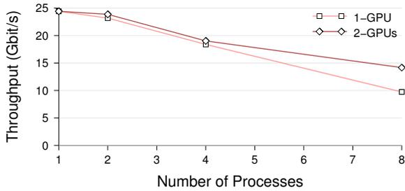
Figure 7: Per-process transfer rate between CPU and GPU.
