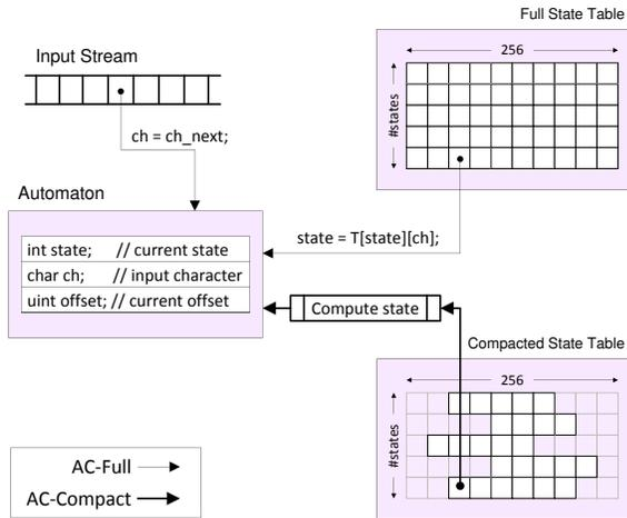
Figure 3: State tables of AC-Full vs. AC-Compact.
