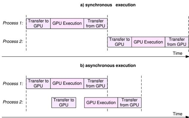
**Figure 5: Data transfers and GPU execution of different processes can overlap.**
