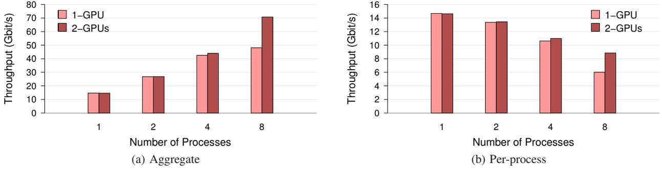
Figure 9: GPU throughput with an increasing number of CPU-processes up to the number of cores.
